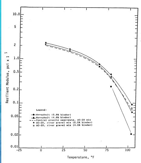
Figure 11. Resilient Modulus Versus Temperature Relationships for Novophalt Mixture Groups (5.8 and 4.8 percent binder) and for Traditional Mixtures Using AC-20 Asphalt Cement without Polyeythelene.
