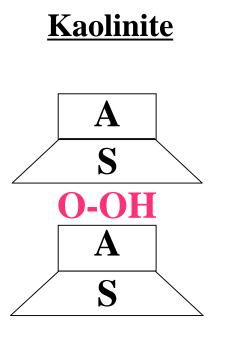
Alumina Sheet Above Silica Sheet O-OH Interlayer Bond = Hydrogen Bond: Very Strong Illite
