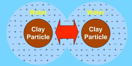
As the water is **adsorbed**, it pushes the clay particles apart, causing an expansion or swelling of the clay.
