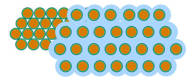
As the water is **adsorbed**, it pushes the clay particles apart, causing an expansion or swelling of the clay.
