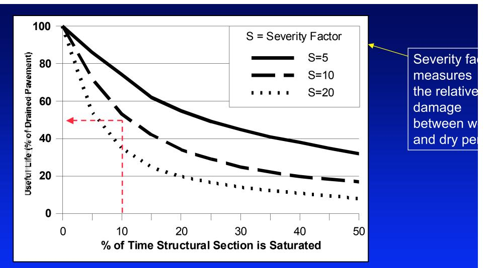
For a pavement section with a moderate severity factor of 10, if 10% of time the pavement is approaching saturation, the pavement service life could be reduced by half.
