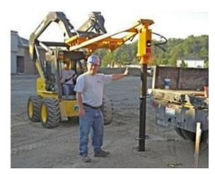
soil conditions. Minimum spacing to avoid group effects is 5D, but 3 ft minimum, where D is the diameter of the largest fin. The Ram Jack helical piles can be used for new construction or repair of foundations. They offer a "Moly Bolt" type of connector for lifting a slab through an interior 10" diameter hole. There is no welding, drilling spoils or vibration during pile installation. Because the piles are torqued to penetration, no structure is needed for reaction resistance during driving.
