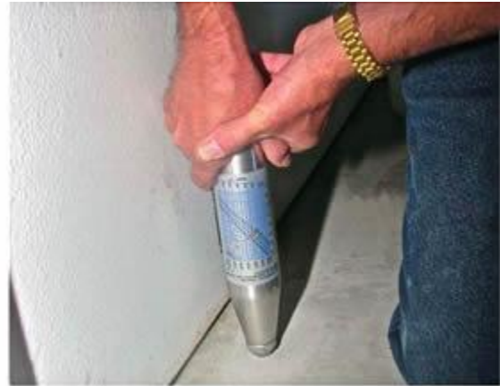
Figure 2.21.1 Rebound hammer testing
