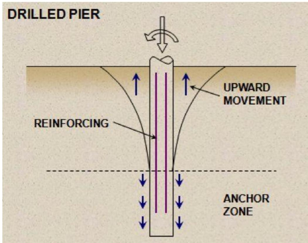
Committee with a scope to develop a method comparable to the Lytton Method that does not require suction testing, but rather utilizes the soil parameters commonly reported in the local market. The design procedure developed allows the sizing of drilled piers to resist movement due to heave and shrinkage.
