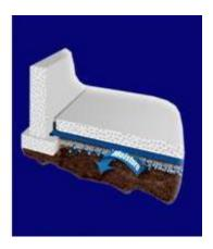
A gas barrier is an impermeable membrane designed to prevent soil gases such as radon, methane and volatile organic compounds (VOC's) from migrating from the soil through concrete and into the building or residence. Gas barriers contain multiple layers that incorporate specific resins designed to block and resist gases. A gas barrier may also be designed to block the migration of moisture.
