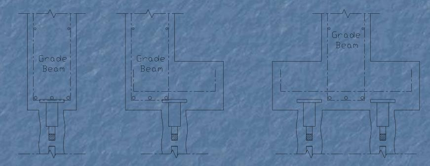
± 3 inches Within Tolerance (3631 Places or 99.6 %) ± 3 to 9 inches Out of Tolerance (14 Places or 0.4 %) > 9 inches Out of Tolerance (0 Places)
