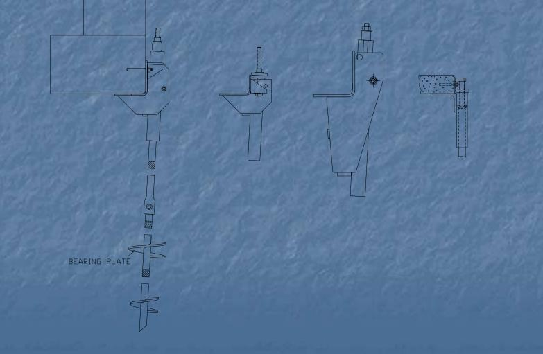
Determining Capacity Helical Anchor/Foundation In soil Soil Borings/Calculations Torque Correlation
