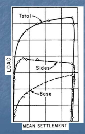
Maximum side resistance (friction) is mobilized after downward displacement of from 0.5 to greater than 3 percent of the shaft (grout column) diameter, with a mean of approximately 2 percent [Reese, Wright (1977)].
