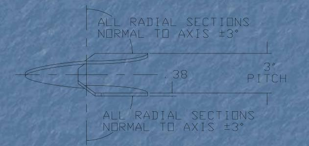
Helix formed by matching metal die so that soil disturbance is minimized.
