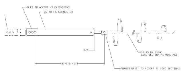
1-1/2 SS to 2-7/8 Pipe 1-3/4 SS to HS (3.5 O.D. x 0.300 Wall) 2 SS to HS 2-1/4 to 4.5 O.D (Atlas) 8" Pipe Shaft to 2" Square Shaft with 3 Helixes
