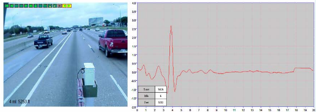
GPR along Edge Side Wheel Path
