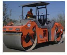
paver and then achieving final compaction and densities with a steel wheel drum roller. Whereas the RCC product is a cementitious concrete, the production and placement process resembles that of asphaltic concrete.
