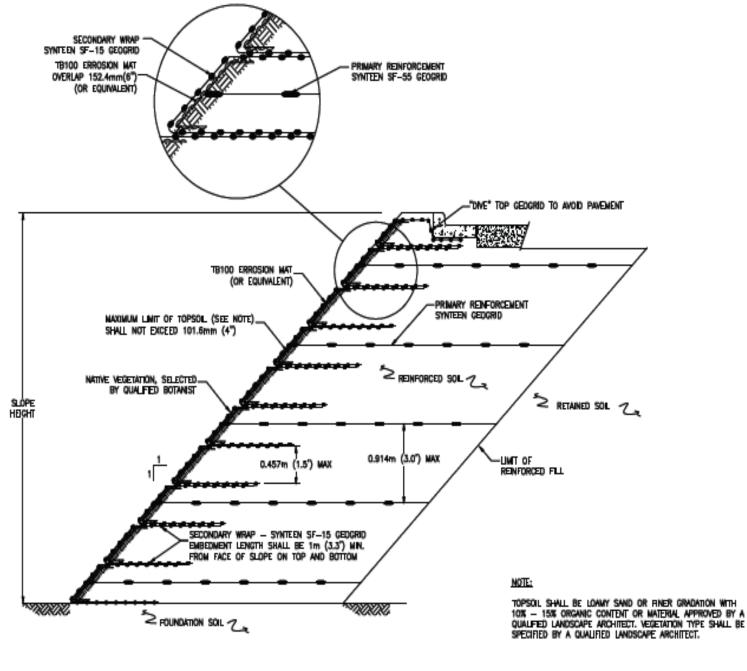
MECHANICALLY STABILIZED REINFORCED SLOPE TYPICAL CROSS-SECTION
