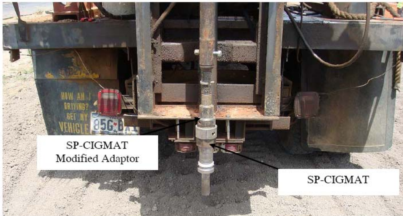
Figure 5. SP-CIGMAT Mounted on a Soil Sampling Rig
