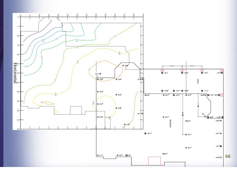
Align the plots so that the contour plot is aligned with the floor plan
