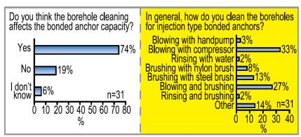
Fig. 13: Many installers were not aware of the influences of significant factors on anchor capacity:
