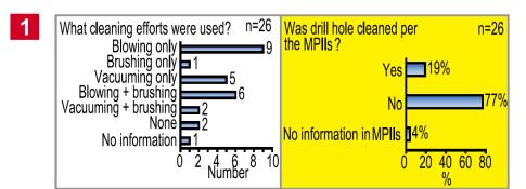
Fig. 2: Results of the field study of adhesive anchor installations. (n = number of observed applications)
