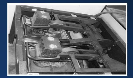
Hamburg Wheel-Tracking Device (HWT<sub>3</sub>)
