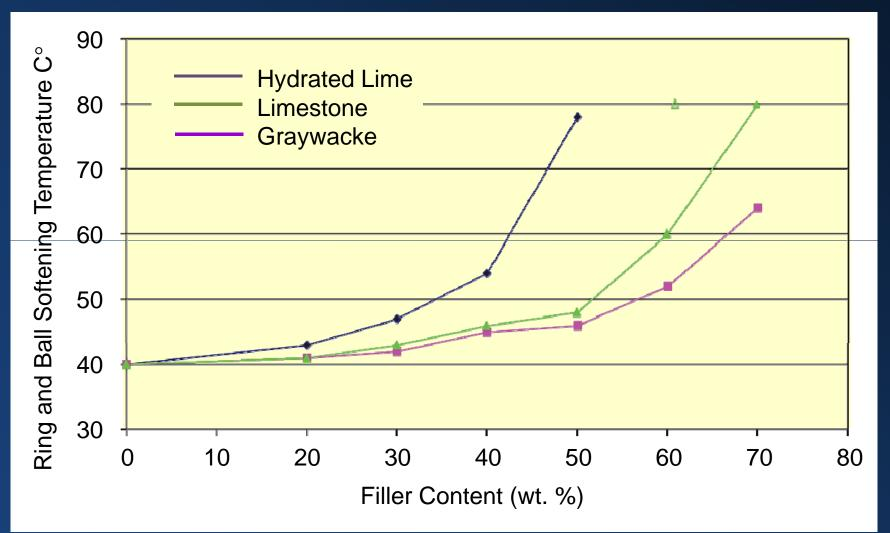
Hydrated lime added to the bitumen has a substantially greater impact in reducing the softening point of asphalt binder than does filler from graywacke or limestone source. Why?
