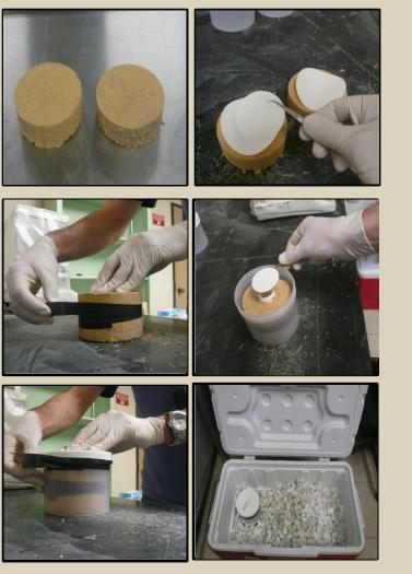
Prepare two generic soil samples by using standard impact compaction machine.
