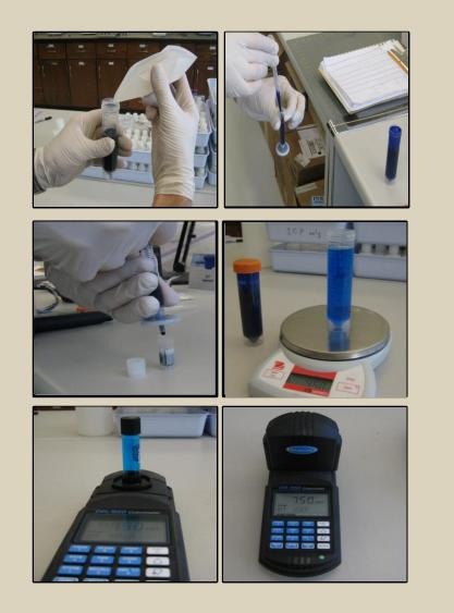
Weigh 20g of sample\*\*\*and 30g MB solution. Mix them and shake for 5 min.
