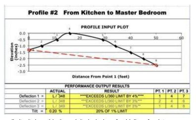
performed within certain foundation performance limits; it does this through its inclusion of guidelines for data acquisition and presentation of the data, coupled with prescribed computations that are compared against limiting movement criteria.
