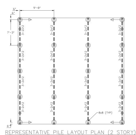
HELICAL PILES (SEE SHEET F3.3) MAY BE INSTALLED IN LIEU OF WOOD PILINGS AT IDENTICAL LOCATIONS.
