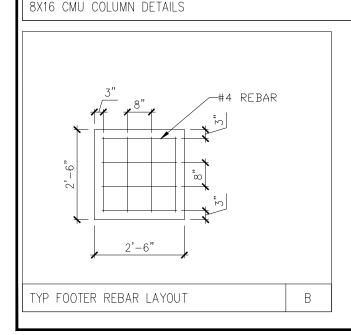
ALL CMU CELLS TO BE FILLED WITH CONCRETE (MINIMUM OF 2500PSI)
