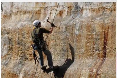
3-lb Impulse Hammer impacts on downstream face for testing on rough surfaces and thick dams
