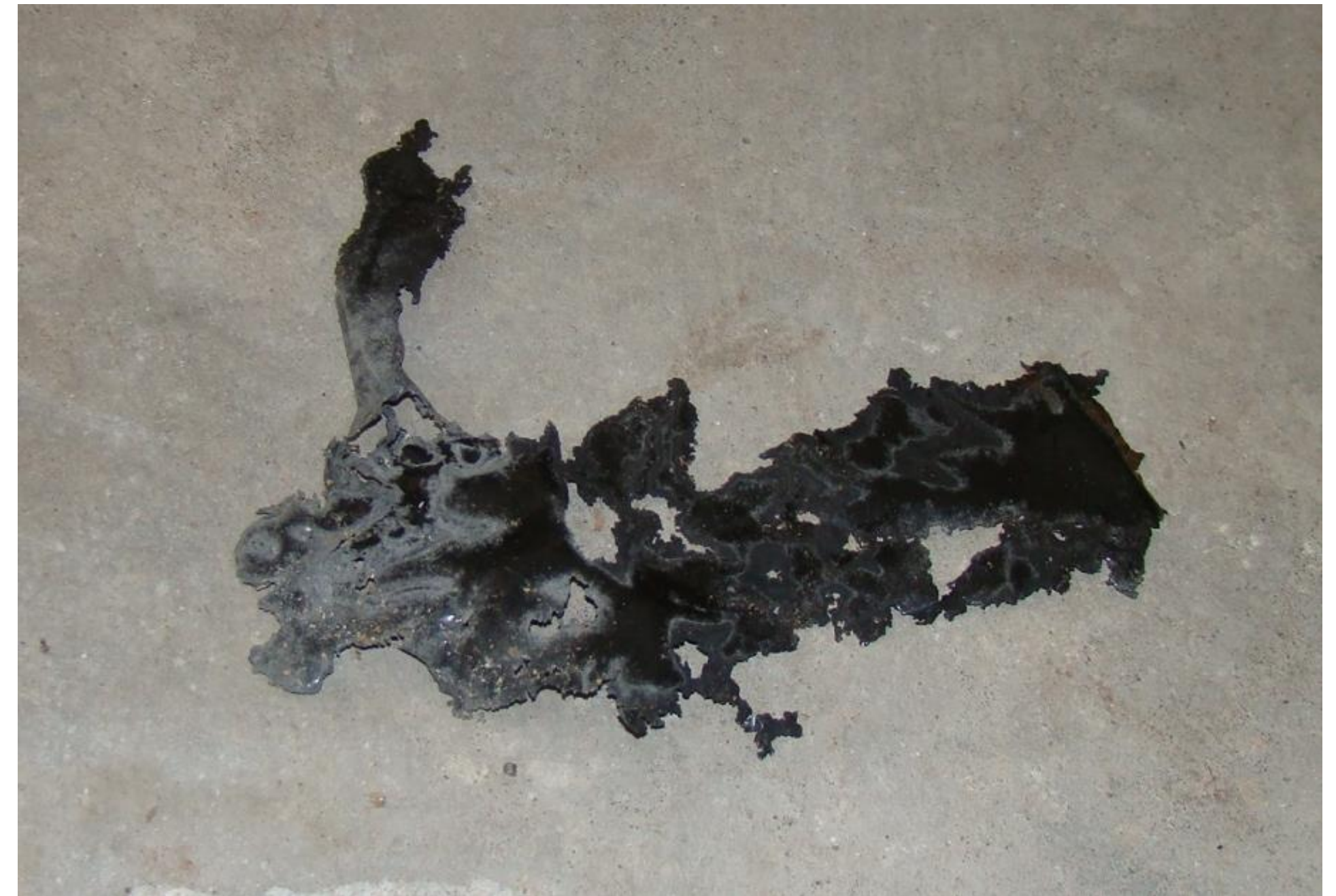
Vapor retarder that deteriorated after 50 years
