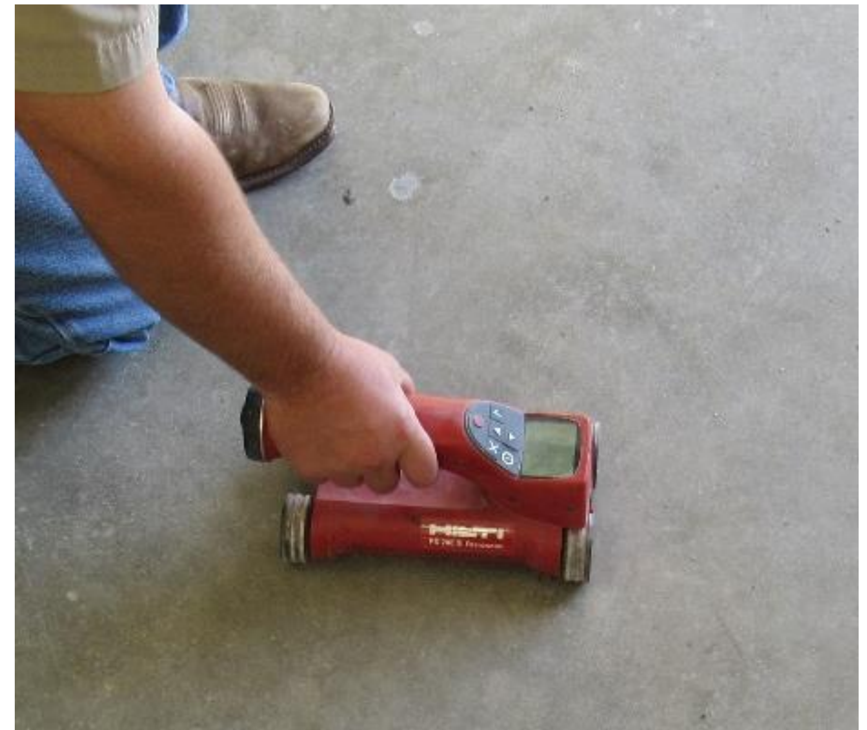
Cover-meter to detect reinforcement
