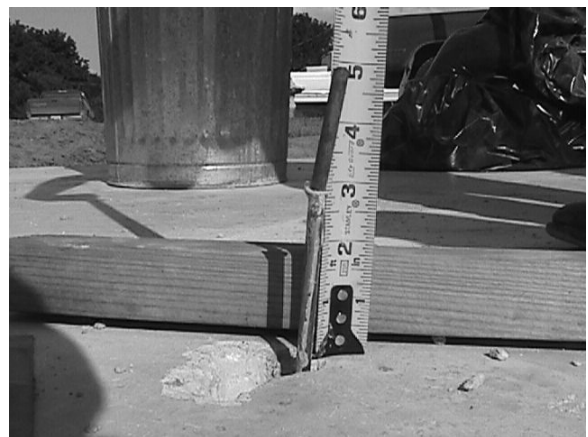
Slab indicators showing the “heaving” of the soil and therefore the failure of the boxes
